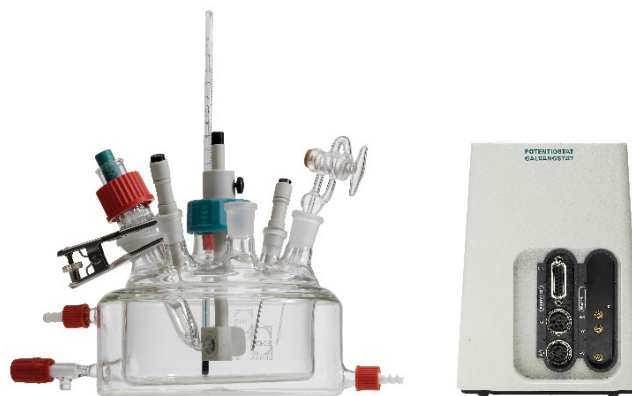
Figure 1 - The 1 L corrosion cell and the PGSTAT204 with the FRA32M module
