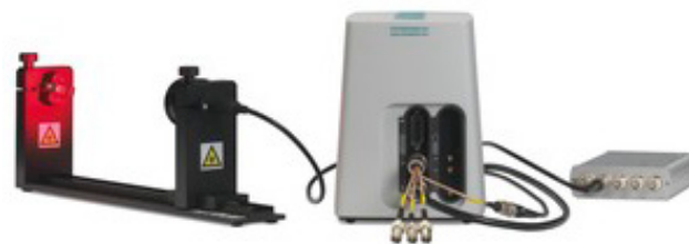
Figure 1 – On the left, the rail equipped with the 627 nm red LED light and the photodiode. In the center, the Metrohm Autolab PGSTAT204. On the right, the LED driver.
