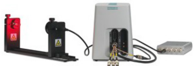
Figure 1 – On the left, the rail equipped with an LED light and the photodiode. In the center, the Metrohm Autolab PGSTAT204. On the right, the LED driver.
