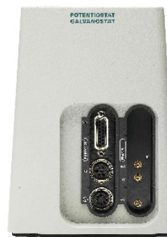
Figure 1 – The Metrohm-Autolab PGSTAT204, with the FRA32M module.
