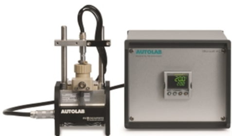
Figure 2 - The Autolab RHD Microcell HC setup, composed of a cell stand (left-hand side), and the temperature controller (right-hand side).
